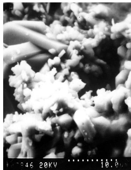
Fig. 3 SEM microstructure of powder synthesized by SHS.
